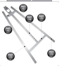
Attach side supports part #3, by slotting onto piece from previous step. Ensure rounded ends of the side supports are at the top. Turn A frame over, drop in barrel nut and insert bolt from side and through barrel nut to secure using (Bag B).
