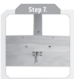
Screw trigger from (Bag E1), to base of accessories tray part #8, into pre-drilled holes as shown.
