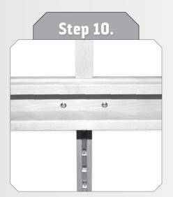
Fix small **C** shaped piece of wood over central A frame column onto accessories tray with nut and bolt from (Baq G) as shown.
